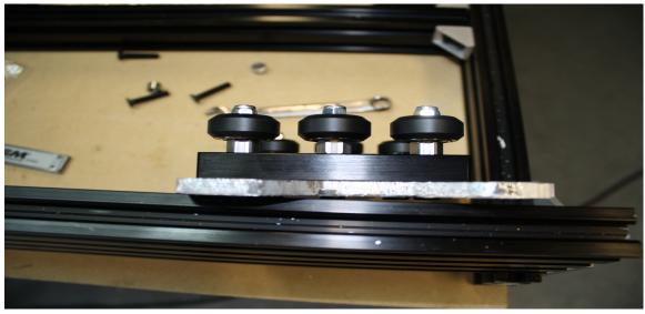
Now install a M5 x 65mm bolt into the front gantry plate. Build a wheel kit. Install the  $\frac{1}{4}$ " spacer, the wheel,  $\frac{1}{4}$ " spacer, a 3mm spacer, another wheel kit and the  $\frac{1}{4}$ " spacer, then the back plate and a nut. Do this for all four top axles on the X gantry. Leave the four M5 nuts loose for now.
