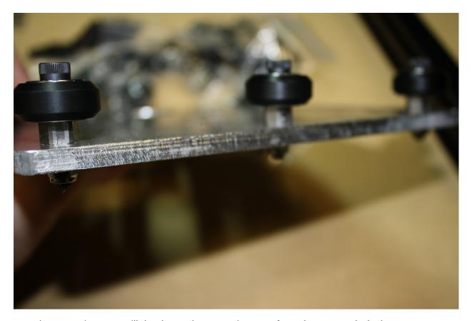
Turn the eccentric spacers till the slot on the eccentric spacer faces down towards the bottom edge of the plate.
