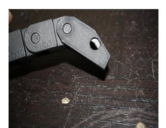
The install the spacer, bolt and nut. Then run all cables through your chain.
