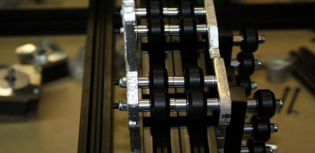
Now install the lower two axles, this time use an eccentric spacer in place of the outside  $\frac{1}{4}$ " spacers.
