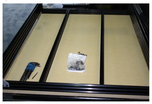
The 20 x 80 rails sit on top of the 20 x 40 rails and form a square. The support rail will be in the center of the box. Note: large format shown above with two cross members, small format only has one.
