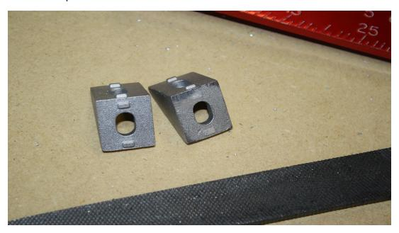
Lay the flat side of the cast 90 (you just filed off the tabs) against the gantry plate and attach it with a M5 nut and M5 x 15mm bolt, do the same for the other side of the gantry.
